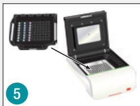
5 Place speed loader tray into instrument.
